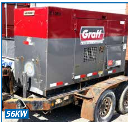
56KW MQ POWER WHISPERWATT DIESEL GENERATOR
