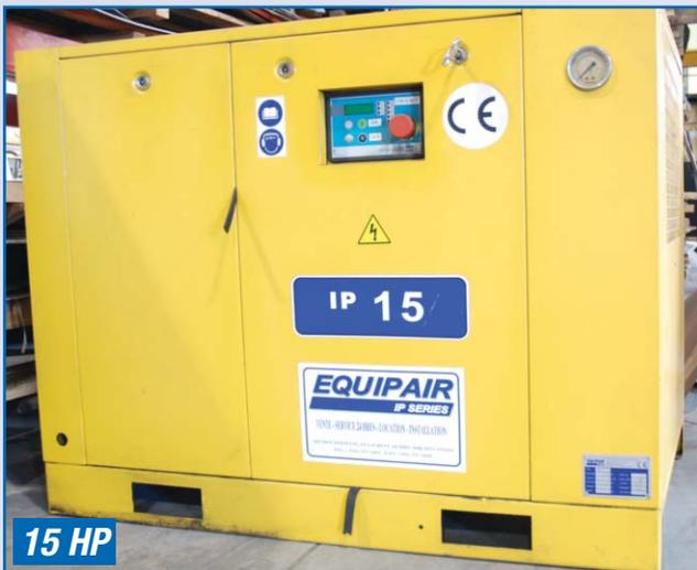
EQUIPAIR ROTARY SCREW AIR COMPRESSOR
