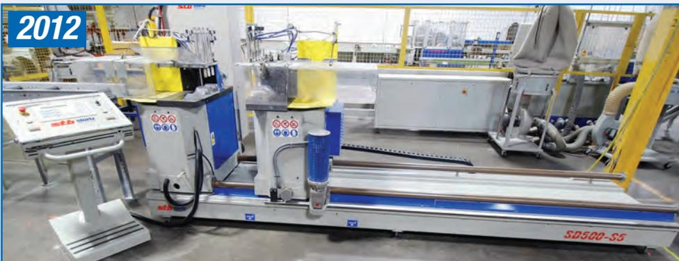
**STURTZ SD500 AUTOMATIC DUAL MITRE SAW, AUTO ANGLE ADJUSTMENT (90 - 45 DEGREE) W/ SELECTOR SWITCH, INDEPENDENT HEAD OPERATION, S/N 28957**
