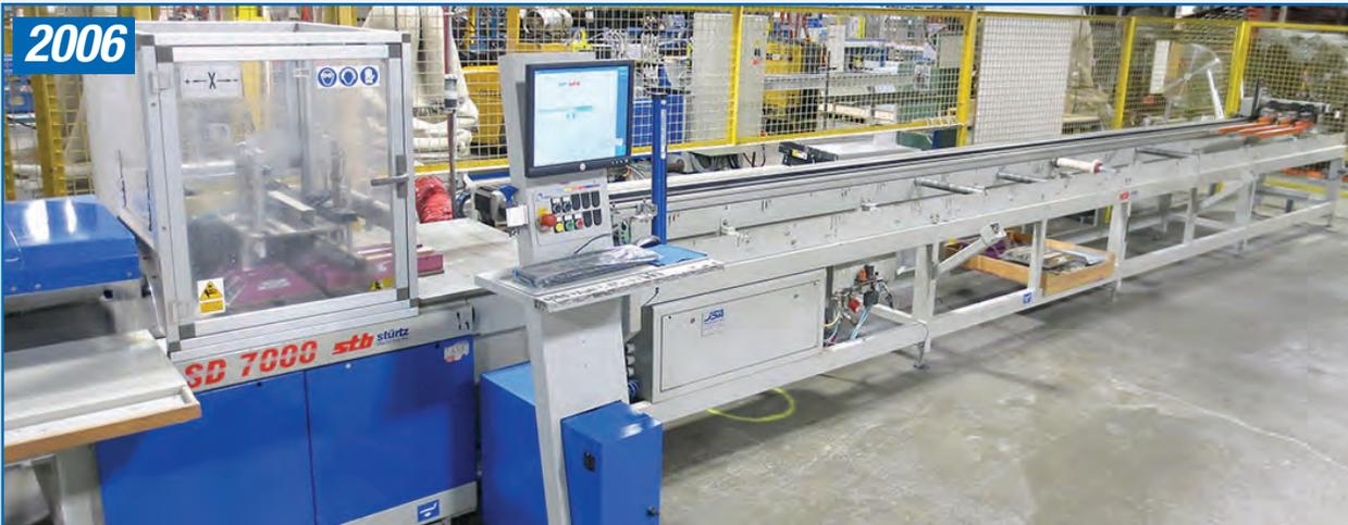
**STURTZ SD7000 AUTOMATIC CNC SAW, 18" X 25' INFEEED TABLE, 2 PLC CONTROL PUSH BAR, 6 CLAMPING CYLINDER, S/N 21133**
