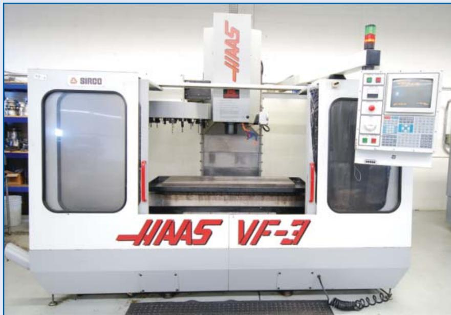
**HAAS VF-3** CNC Vertical Machining Center, With HAAS CNC Control, 18" X 48" Table, Travels: X-40", Y-20", Z-25", Cat 40, 4th Axis Ready, 7,500 RPM, 24 ATC, 15 HP High Torque, Programmable Coolant, 208/230 Volt 3 Phase, S/N 5325
