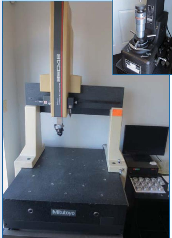
**MITUTOYO B504B** CMM With Travels X-20", Y-16", Z-12", Computer And Interface, Code 195-121, s/n 9110010
