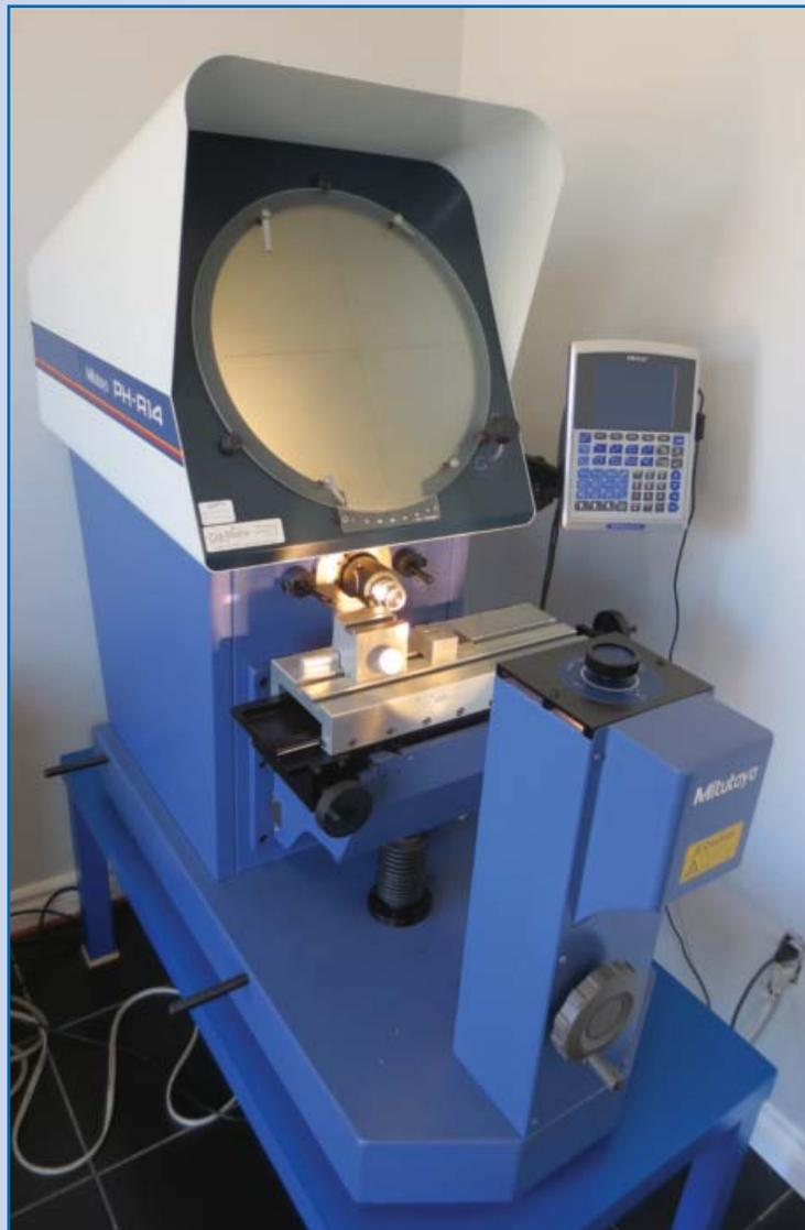
**MITUTOYO PH-A14** Optical Comparator With QM-Data 200 Readout, 14" Screen, 8" X 4" Travel, 100 Lbs. Cap., Linear Glass Scales, Code 172-810A, s/n 605014
