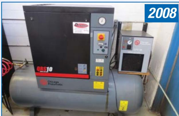
**CHICAGO PNEUMATIC QRS10** Rot. Screw Air Comp. W/ Tank, With CHICAGO CPX 60 Air Dryer
