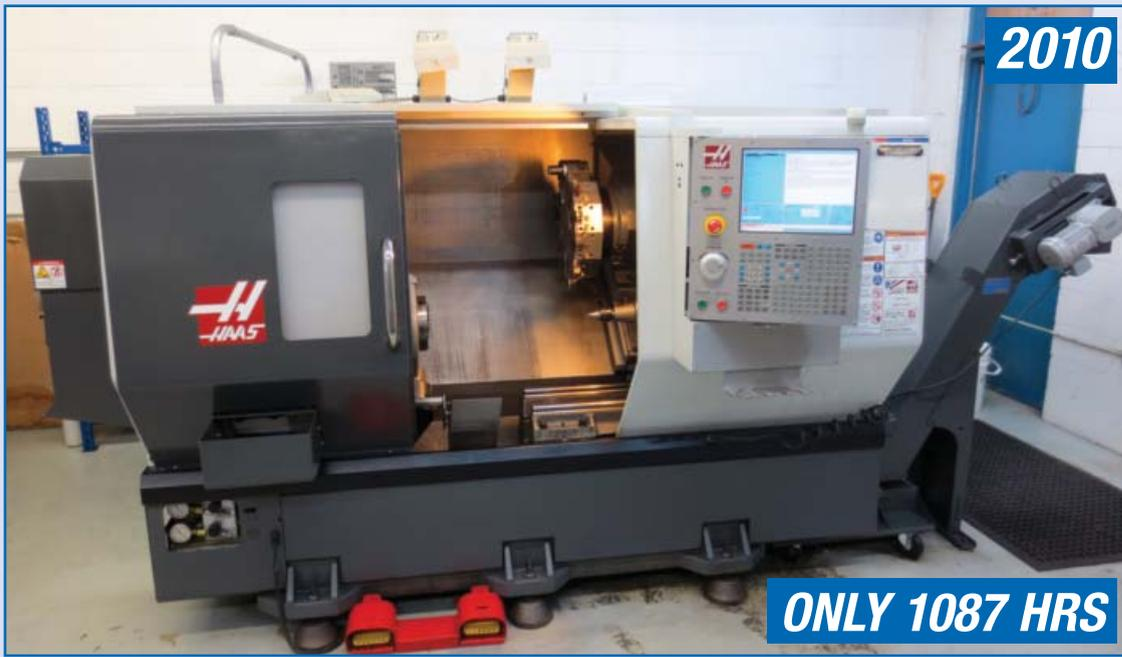
2010 **HAAS** ST20 CNC lathe With HAAS CNC Control, 8" 3 Jaw & 6" 3 Jaw Chucks, 15" Swing X 23" Between Centers, 2" Bore, 4,000 RPM Spindle, 20 HP, 12 Station Turret, Tool Presetter, Parts Catcher, 2 Worklights, Coolant, Chip Conveyor, 195/260 Volt, 3 Phase, s/n 3085784 \***Only 1,087 Cutting Hrs.**
