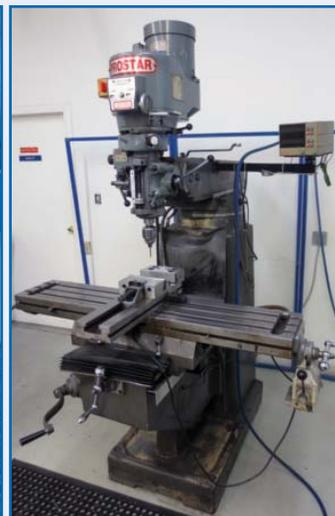
1997 **PROSTAR M-3S** 3HP Vertical Mill With Dro, Power Feed
