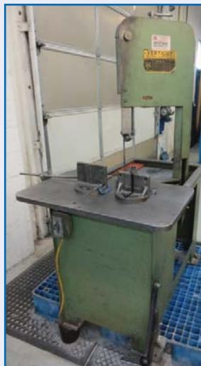
**VERTICUT 115B** Roll In Bandsaw With 10" X 13" Cap., 13" Throat, S/N 372
