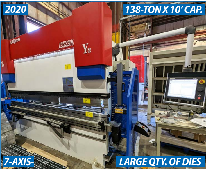
ADH WAD-125T/3200 CNC HYDRAULIC PRESS BRAKE
