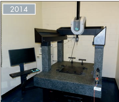
HEXAGON TECHNOLOGY COORDINATE MEASURING MACHINE, MODEL 7.10.7 SF
