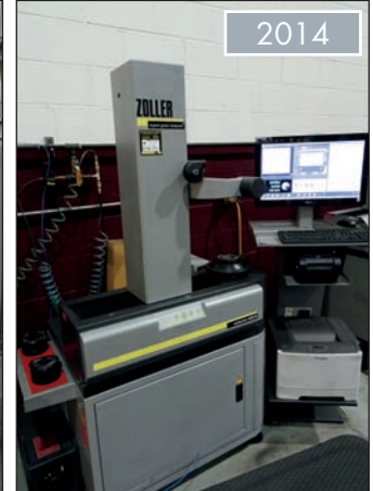
ZOLLER VENTURION MODEL 450/6/D400 CNC TOOL PRESETTER
