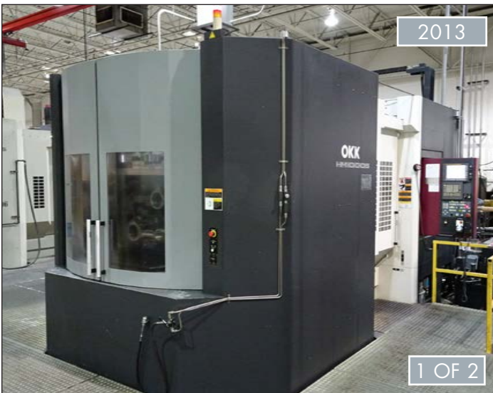
OKK CNC HORIZONTAL MACHINING CENTER, MODEL HM 1000S
