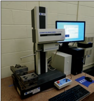
ZEISS CONTOUR RECORD CONTOUR & SURFACE MEASURING MACHINE, MODEL 1710-SD3-13
