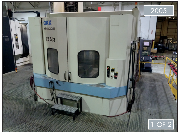
OKK CNC HORIZONTAL MACHINING CENTER, MODEL HM100S
