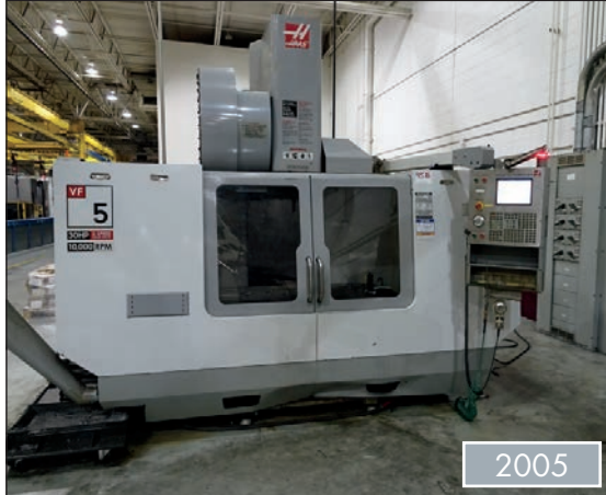
HAAS CNC VERTICAL MACHINING CENTER, VF5/50
