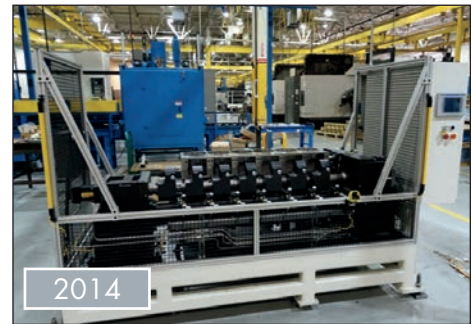
NORTH TOOL CAM BEARING PRESS
