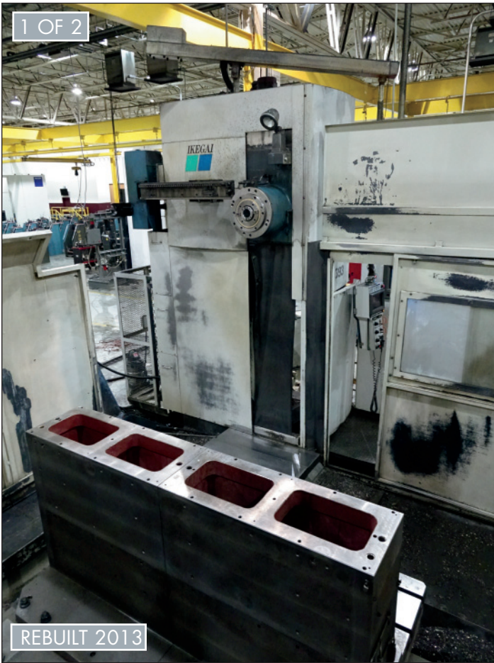
IKEGAI 4" CNC HORIZONTAL BORING MILL MODEL NB110T
