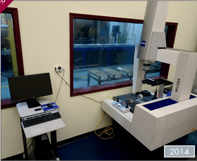
ZEISS COORDINATE MEASURING MACHINE, MODEL MICURA 5/5/5
