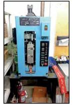
MINI-JECTOR MDL. 551 BENCH TOP LAB INJECTION MOULDER
