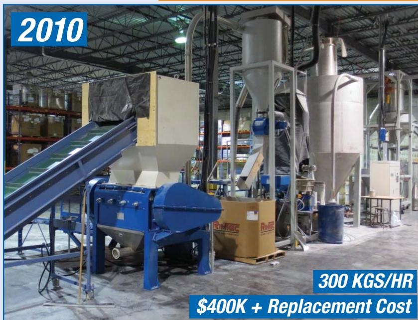
PVC/PLASTICS PULVERIZER AND GRINDING SYSTEM
