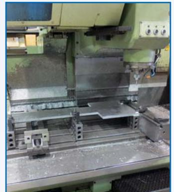
**OKUMA MC-6VA**, Okuma OSP 500M-G CNC control, table size 24" x 60", 50 taper, 20 sidemount ATC, sn 0105 0417
