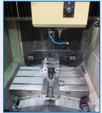
**HITACHI SEIKI VM40II**, Seicos CNC control, travels: X-22.05", Y-16.14", Z-16.14", table size 16" x 30", distance from spindle to table 5.9"-22.05", 8,000 RPM, 40 taper, 20 internal sidemount ATC, tapping, flood coolant, chip auger, sn 42251
