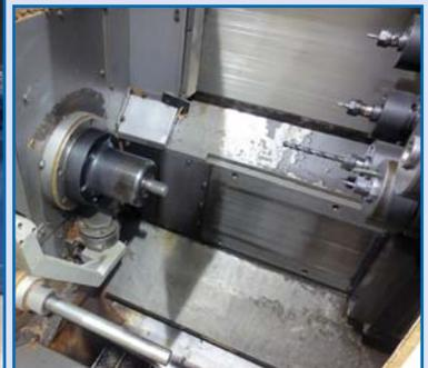
HITACHI SEIKI HT20SII, COLLET CHUCK HITACHI CNC CONTROL, 10 STATION TURRET, TAILSTOCK, TOOL PRE SETTER, PARTS CATCHER, CHIP CONVEYOR, 5,000 RPM, SN HTS 221471
