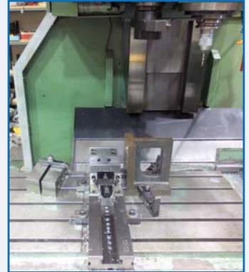
**KURAKI KV-1000**, Fanuc 6M CNC control, travels: X-41.34", Y-23.62", 55" x 24" table, 50 taper, 24 ATC, sn 10026
