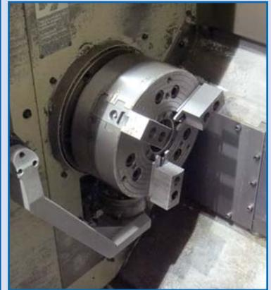
HITACHI SEIKI HT23SII, 10" 3 JAW CHUCK HITACHI CNC CONTROL, 10 STATION TURRET, TAILSTOCK, TOOL PRE SETTER, 3,600 RPM, SN HTS 2746HL
