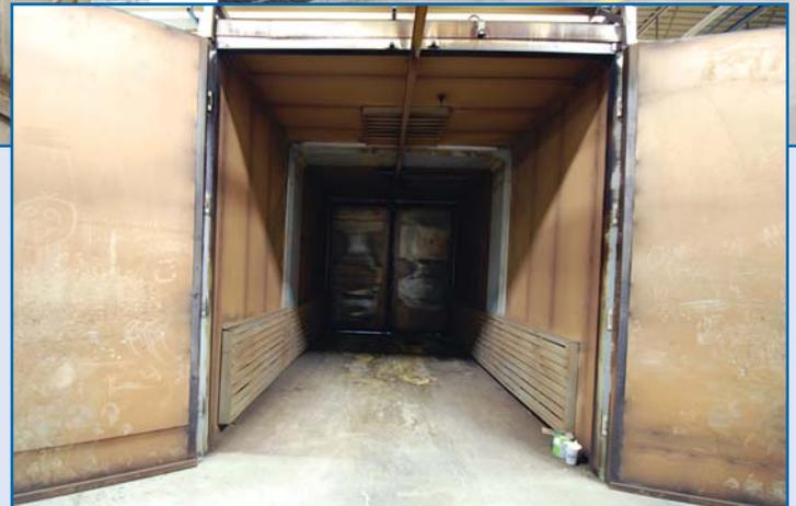
**ELECTRO SOLUTIONS/FILCO** Pass through wash/dry combination booth with 13ft W x 11ft H opening x 50ft length, 1.5M BTU oven ref# 325-06-A / 330-02A
