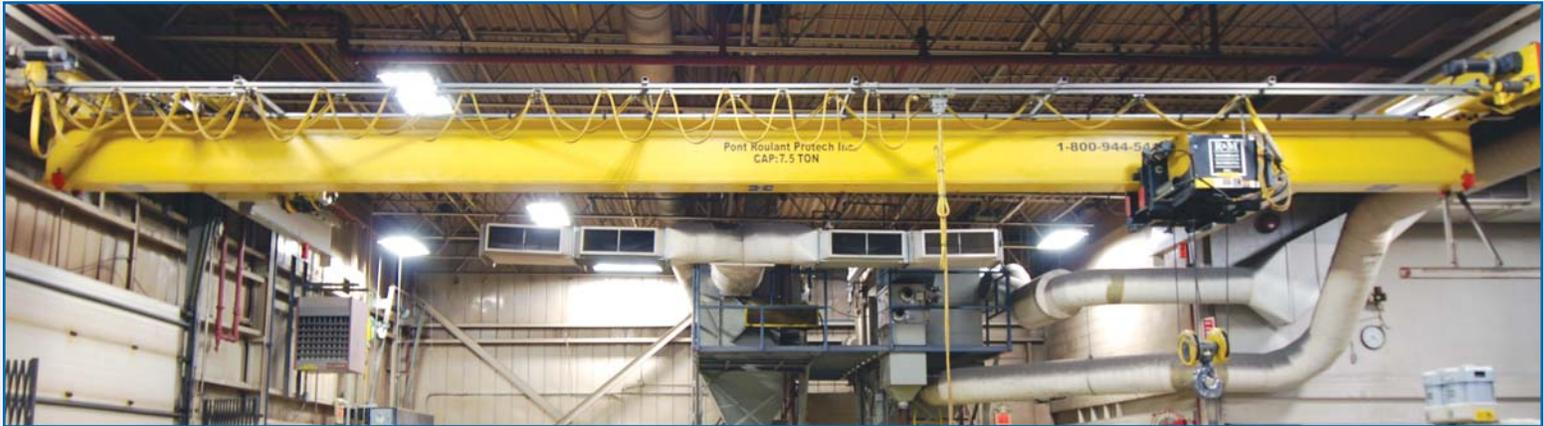
**PROTECH 7.5 TON** single girder underslung overhead bridge crane with approximate 37.5 ft. span, R&M SPACEMASTER SX 7.5 TON underslung hoist with pendant control s/n 915-22-A
