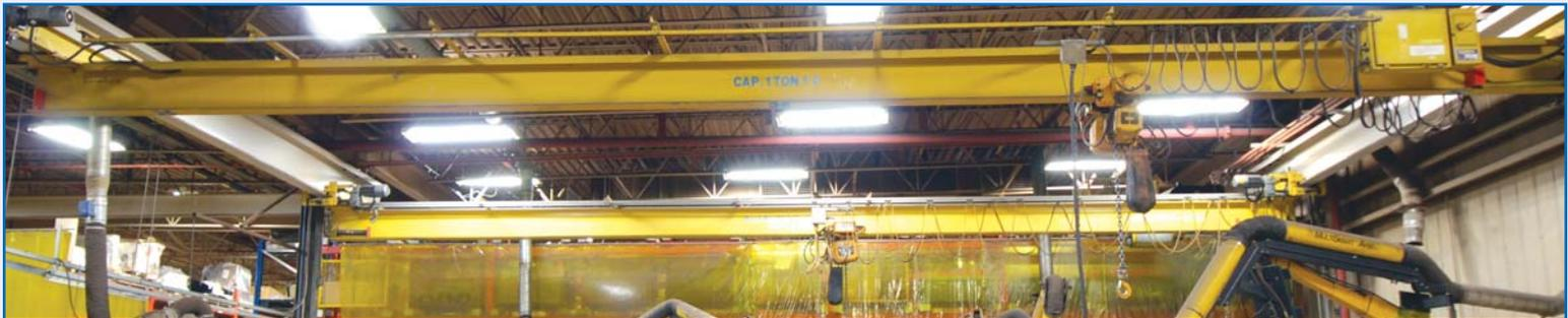
**(2) PROTECH 1.5 TON** single girder underslung overhead bridge cranes with approximate 37.5 ft. span, KITO 1.5 TON underslung hoists with pendant control
