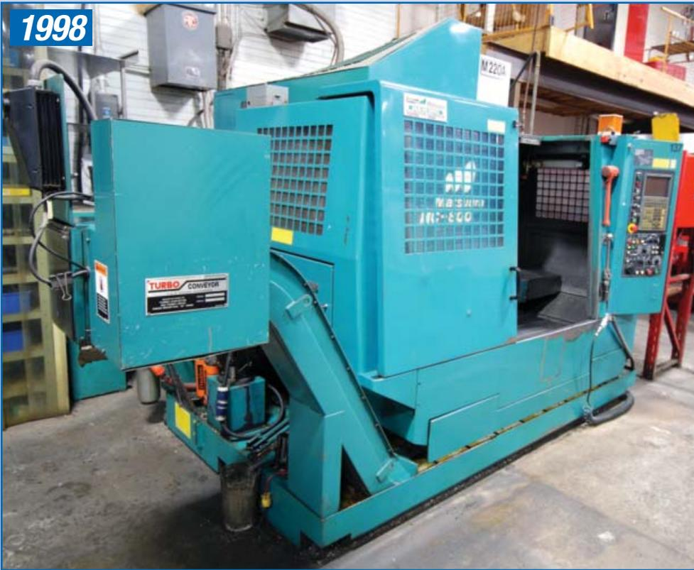
1998 **MATSUURA** MC-800VG CNC Vertical Machining Center With Yasnac CNC Control, 20" X 45" Table, Travels: X-31.5", Y-20", Z-20", Bt-40 Taper, 24 ATC, Chip Conveyor, 10/15 HP, 200/220 V, 3 Phase s/n 980313360
