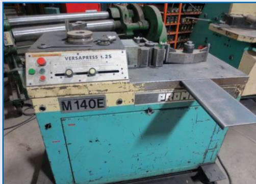
**PROMECAM** 25 ton horizontal **VERSAPRESS** with 17" stroke, 31.5" x 23.5" work area
