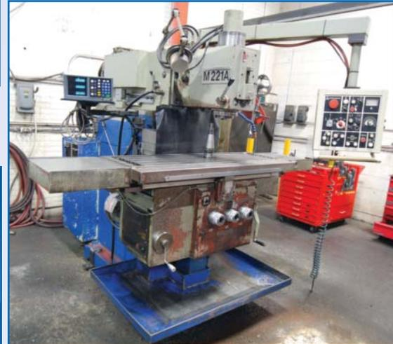
**TOS** Vertical Mill With 15.75" X 55" Table, 1,800 RPM, Power Feeds, With DRO
