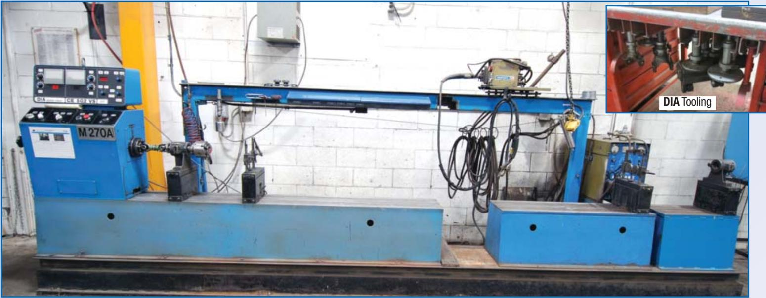
**DIA CE 502 VS Electronic Dynamic Balancing Machine With 450 RPM For Shafts And 900 RPM For Propeller Shafts And Rotors, Weld Unit, Large Qty Of Attachments And Tooling s/n 10182**
