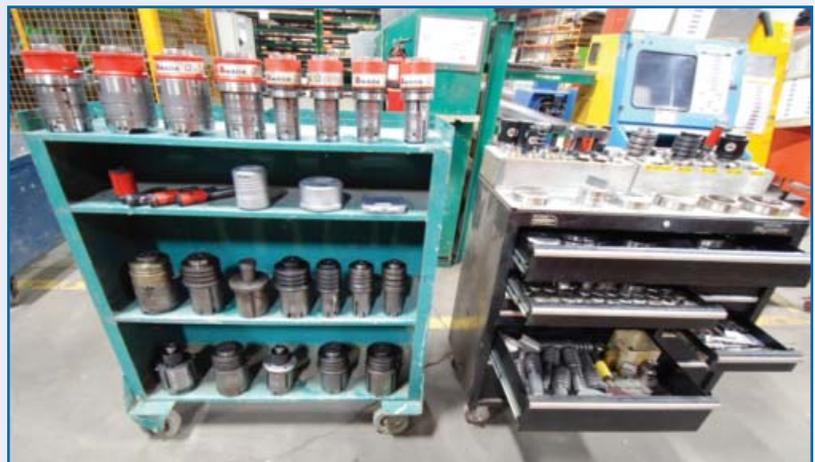
QTY of **AMADA MATE, Z-TOOLING, AIR BLOW, WILSON** (Station A, B, C, D & Multi-Tool) Tooling for Turret Punch
