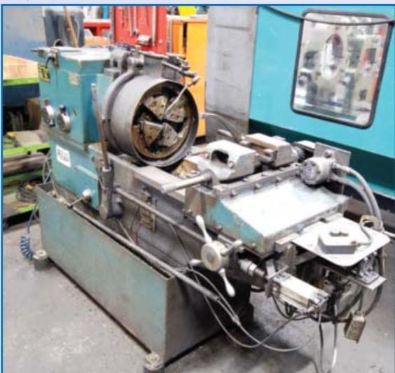
**JOSHUA HEAP** Power Threader With Up To 3" Capacity s/n 965T
