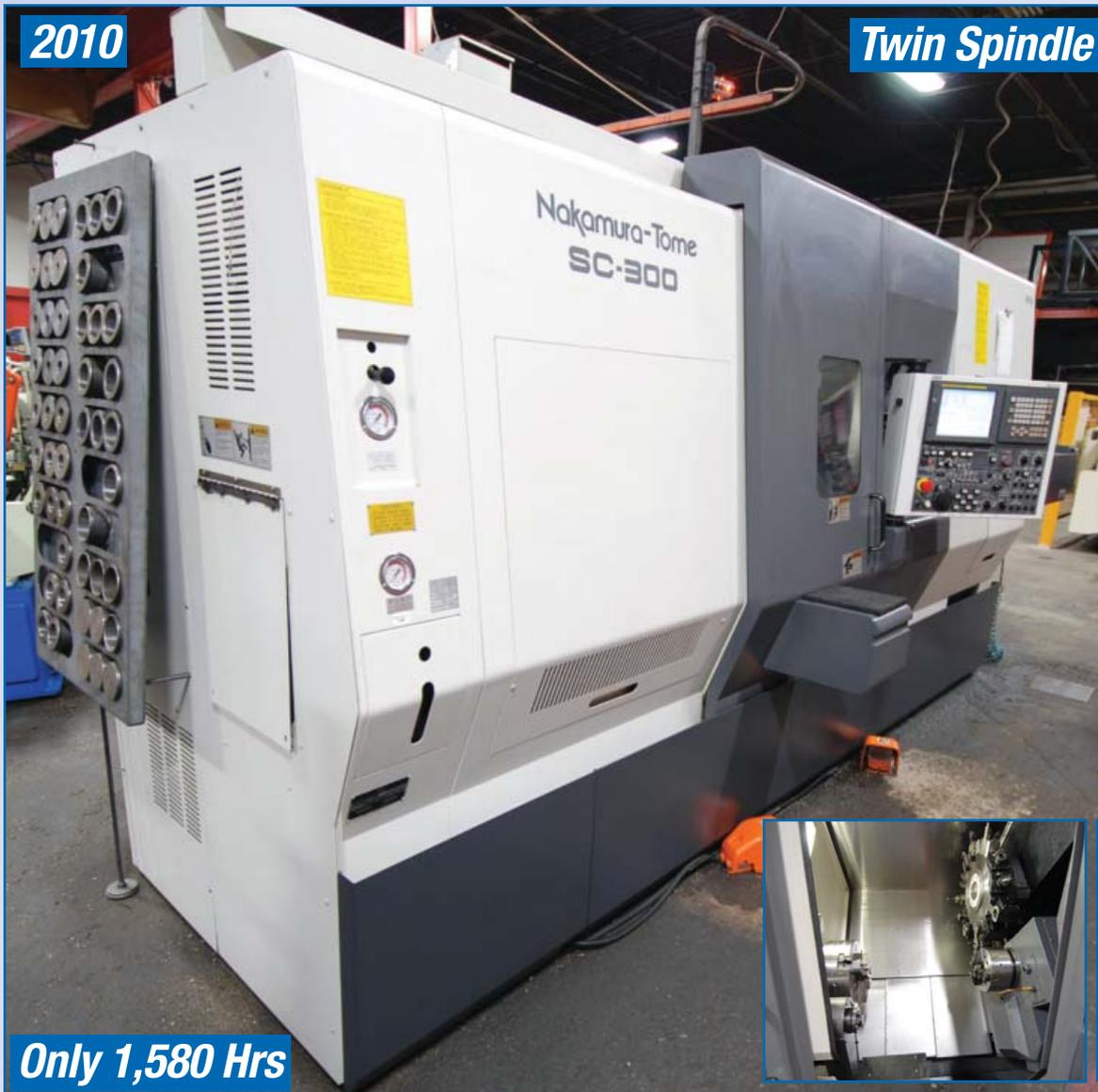
2010 **NAKAMURA - TOME** SC300 twin spindle CNC lathe with FANUC 18iB CNC Control (Upgraded 10.4" Color Screen), 13.78" Max Turning Dia., 31.89" Distance Between Opposed Spindles, Travels: X-8.76", Z-25", B-19.66" (Sub Spindle), 2.80" Bar Cap., 12" Main Spindle Chuck With 3,500 Rpm, 8" Opposed Sub Spindle Chuck With 3,500 Rpm, 12 Station Turret With Live Tooling, Tool Presetter, Parts Catcher, Chip Conveyor, **KISAGE** Coating On Slides, (Only 1,580 Hrs., Great Condition) s/n S311005
