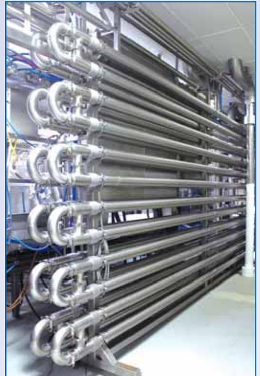
WCB 12-PASS TUBE IN TUBE PASTEURIZER
