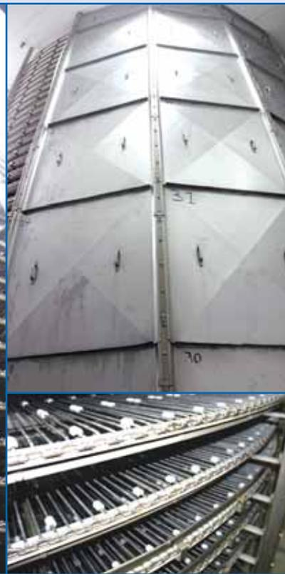
TECHNOPOOL BOLTED FRAME SPIRAL FREEZER – 37 TIER, 36" WIDE BELT, 7" TIER CLEARANCE, BOLTED FRAME, APPROX 22' DIAMETER WITH COOLING UNITS AND CONTROLS
