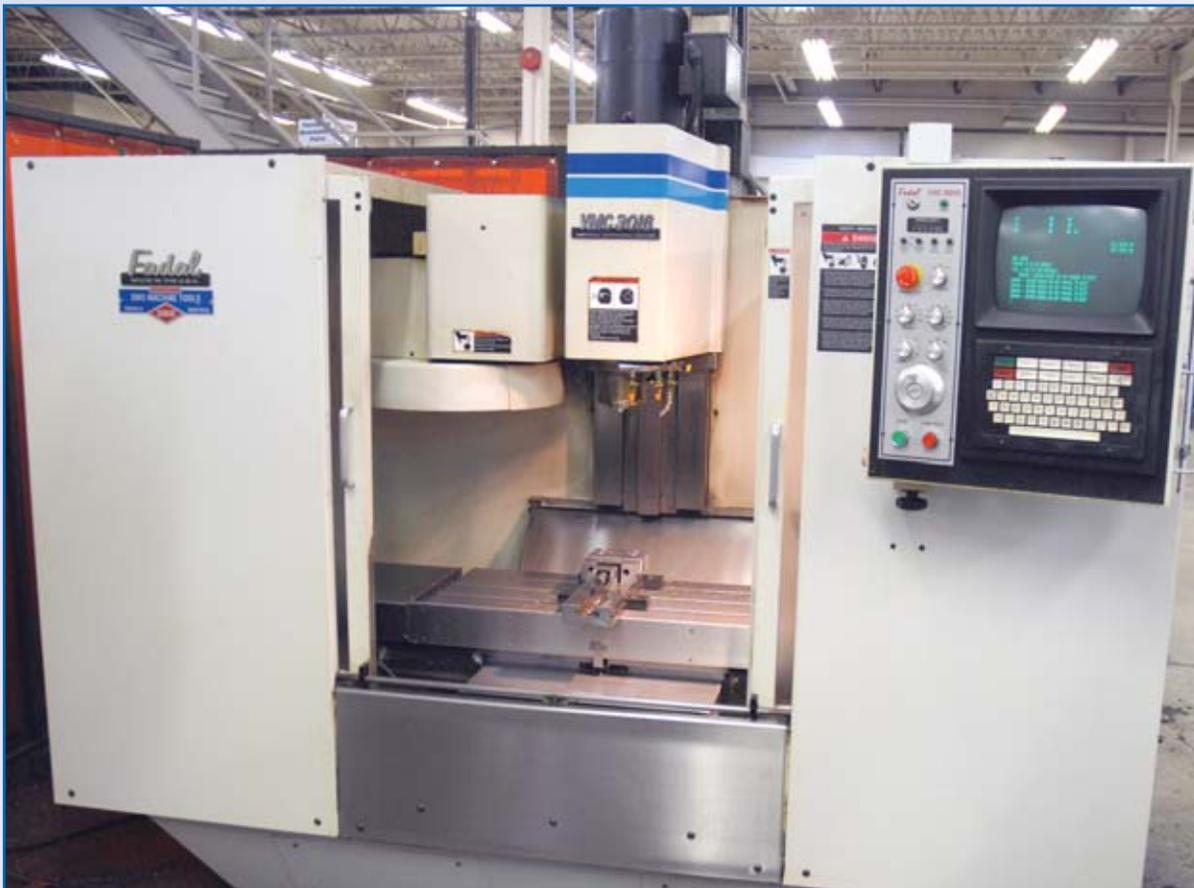
**FADAL VMC 3016**, Model 904-1, CNC 88 HS Controls, Travels: X-30:Y-16", Z-20", Table Size 16"x39.5" Table, Cat 40, 21 ATC, Flood, Mist, RS232, 230/440V, sn 9701909
