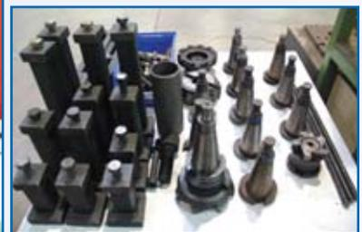
Partial View Boring Mill Tooling, Hold Downs
