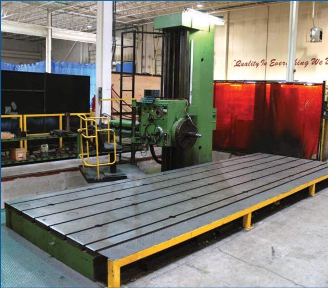
**TOS Floor Type, Model HP 100,** Acurite 3 Axis DRO, Pendant Controls, Table Size 74"x152" (6'2"x21'), Travels: X-240", Y-80", Z-36", 50 Taper, 4" Spindle, Face Head Diameter 24", Max Spindle Speed 1,120 RPM, Max Facing Head Speed 224 RPM, Power Drawbar, Spindle Support, Rapid Traverse 112 IPM, Coolant, 575V, sn 014-13
