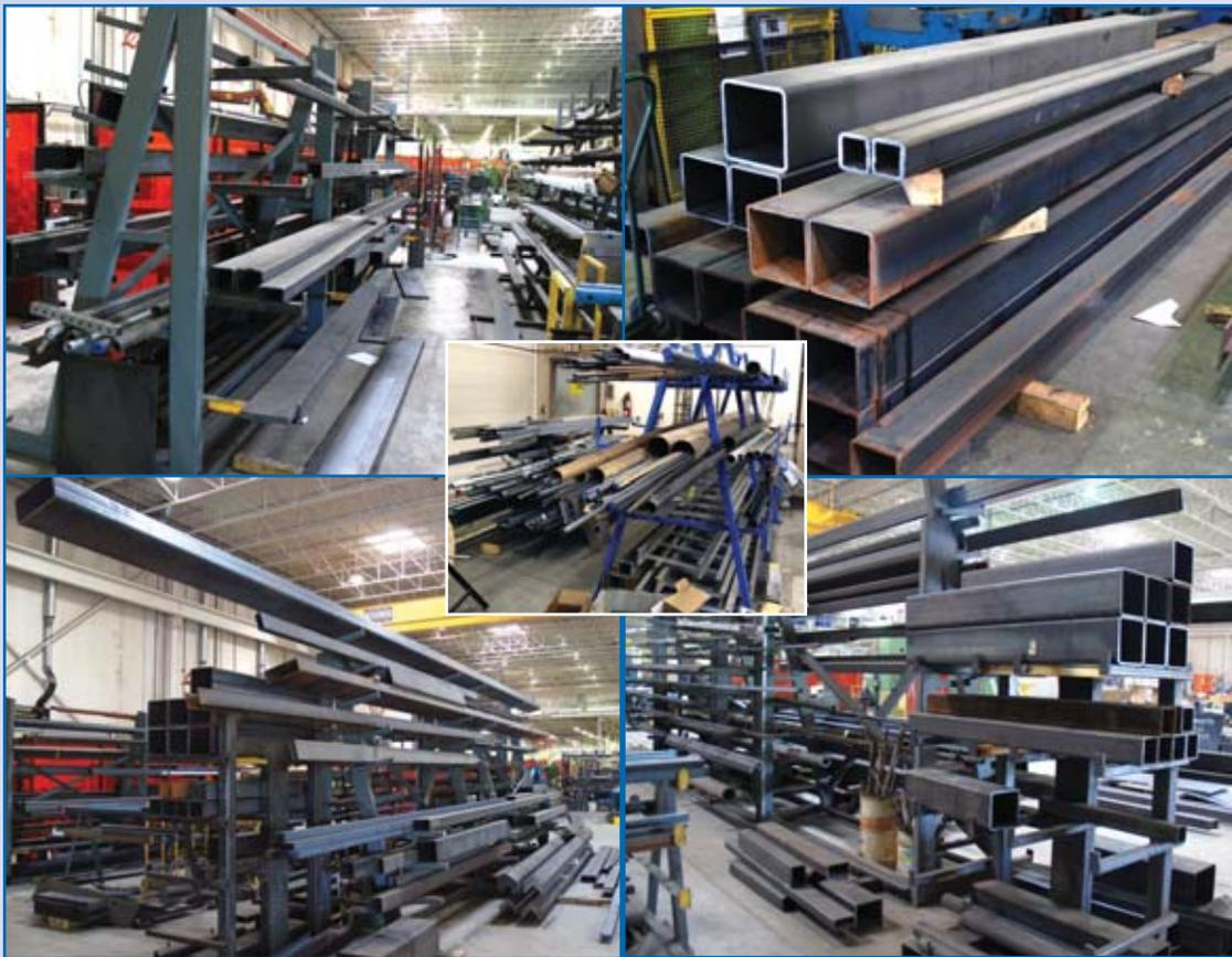
PARTIAL VIEW OF STRUCTURAL STEEL RAW MATERIAL
