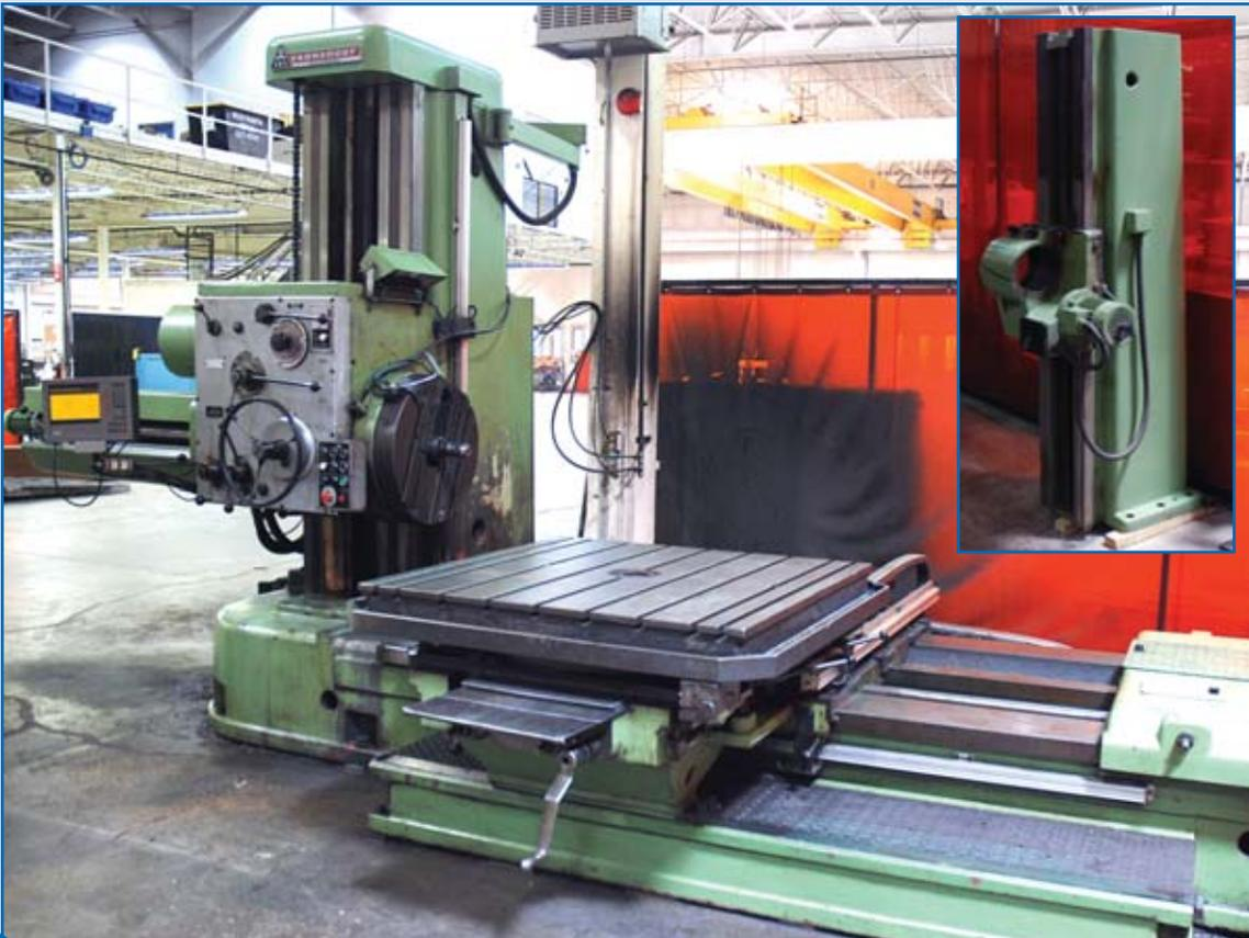
**TOS Model W100A,** Heidenhain Positip 855 4 Axis DRO, Pendant Control, Rotary Table Size 49"x49", Travels: X-63", Y-49", Z-35", W-44", 50 Taper, 4" Spindle, Face Head Diameter 24", Max Spindle Speed 1,120 RPM, Power Drawbar, 5' Tailstock, Max Table Load 6,614 lb, Rapid Traverse 110 IPM, Coolant, 15 HP, sn 09-76
