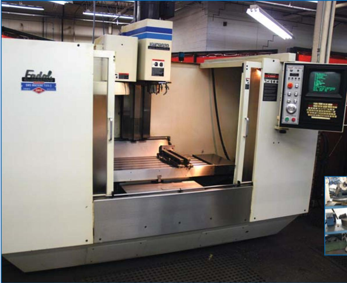
**FADAL VMC 4020HT**, Model 906-1, CNC 88HS Controls, Travels: X-40" Y-20" Z-20" Table Size 47.94" x 20", Max Spindle Speed 10,000 RPM, Cat 40, 21 ATC, Max Table Load 1,500 lb, Rapid Traverse X&Y 700, Z-600 IPM, Flood, Mist, RS232, 15 HP, 230/440V, sn 9606761
