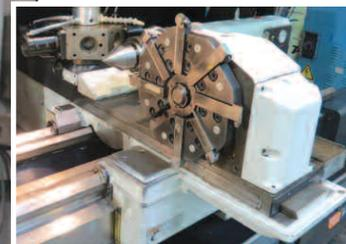
• (2) 2007 MAZAK M-5N-2000 Flat Bed CNC Lathes, Mazatrol 640T Control, Travels: X-22.1", Z-80.9", W-5.1", 4.1" Spindle Bore, 24" Swing, 81.9" Max Turning Length, 24" Chuck, 2,200 RPM, Horiz. & Vert. Turrets, 8 Station Turret, 6 Station Chucker, Tool Eye, Steady Rest, Chip Conveyor, 30 HP, sn's 198318 & 195906
