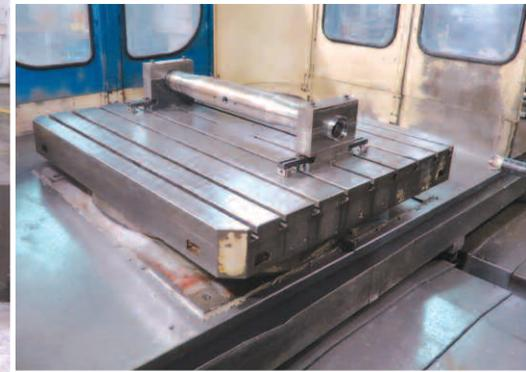
• 1995 TOSHIBA BTD-110R16 5-Axis CNC Table Type Horizontal Boring Mill, Tosnuc 888 Control, Travels: X-98.4", Y-71", Z-57", W-19.7", 4.33" Spindle, 55"x63" Rotary Table, Table Index 0.001", 60 ATC, Cat 50, 2,500 RPM, Rapid Traverse 394 IPM, Table Load Capacity 13,860 lbs, Coolant Through Spindle, Chip Conveyor, Vertical Head Attachment, 40 HP, sn 143590
