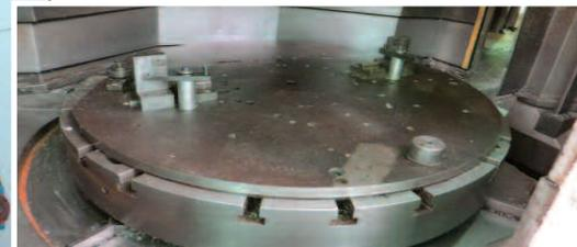
• MAZAK Megaturn A-12 CNC Vertical Turning Center, Mazatrol T32-2 Control, 49.2" Chuck, 57.1" Max Swing, 48.2" Max Height Under Rail, 48" Max Cutting Height, 350 RPM, 16 ATC, Coolant Through Spindle, 30 HP, sn 90796
