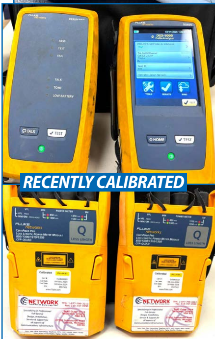
PARTIAL VIEW OF FLUKE VERSIV DSX-5000 CABLE ANALYZERS AND OPTIFIBER PRO QUAD OTDR FIBER OPTIC CABLE TESTING TOOLS
