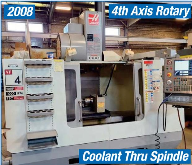
HAAS VF-4B CNC VERTICAL MACHINING CENTER
