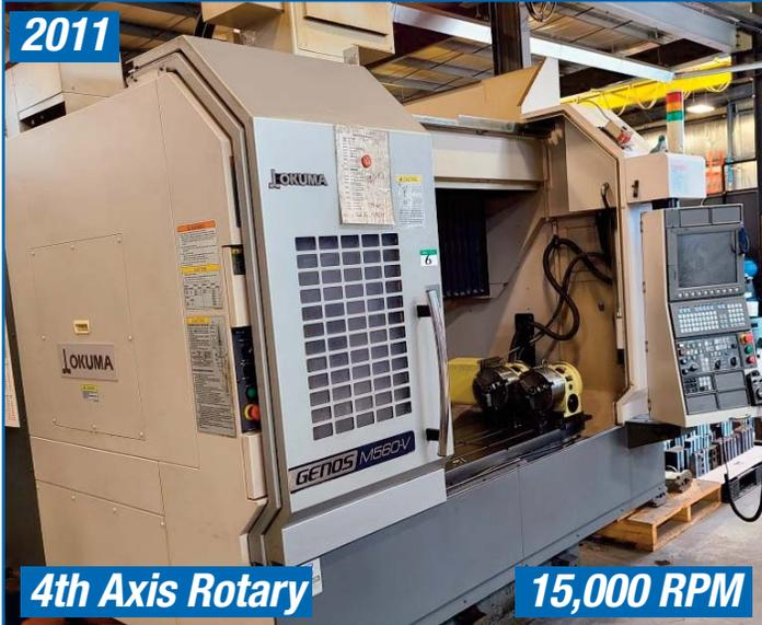
OKUMA GENOS M560-V CNC HIGH SPEED VERTICAL MACHINING CENTER
