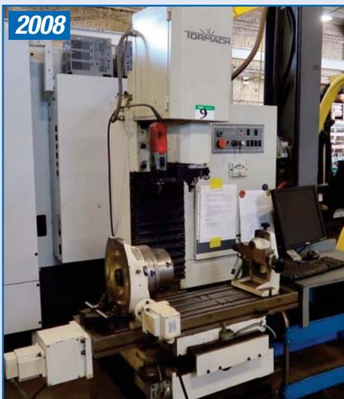
TORMACH PERSONAL CNC 1100 CNC VERTICAL MILLING MACHINE
