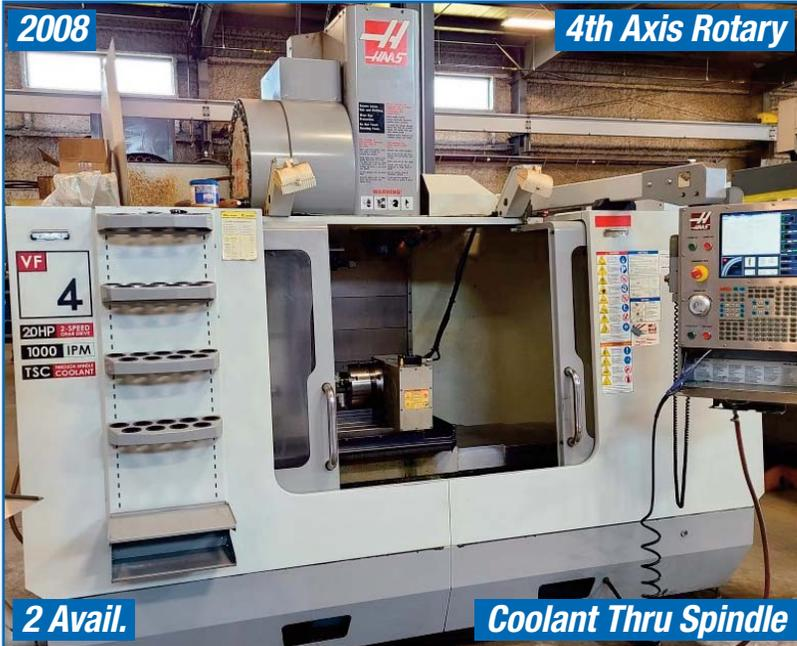
HAAS VF-4B CNC VERTICAL MACHINING CENTER
