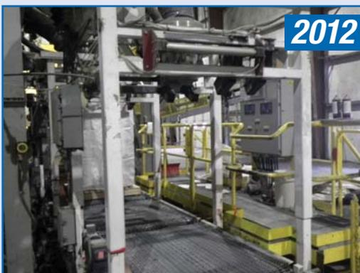
2012 Semi-Automatic Bulk Bagging Line Model 10-DG-001 Including Pallet Feeder, TWO - Custom Equipment Design Model BB4PWD-396 Bag Loading Stations (s/n's 12-1510 and 12-1509) with Idler Station In-Between, Bag Inflation Blowers, Auto Fill Stop, Auto Pallet Advance and TWO Powered Pallet Discharge Conveyors w/ Control Panel w/ Dual Mettler-Toledo Digital Scales 119
