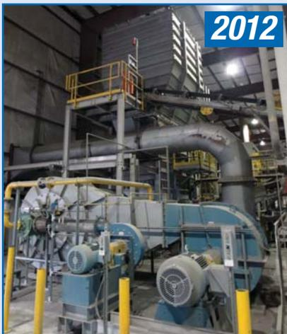
2012 Thermal Kinetics Model TKCFB 11.5-6 Fluid Bed Dryer, s/n MGCA-11228, Natural Gas Fired, 14,000,000 BTU c/w 40 HP Combustion Fan & 125 HP Blower Fan c/w Baghouse Assembly, Exhaust Fan & Stack (Cost \$750,000 USD)
