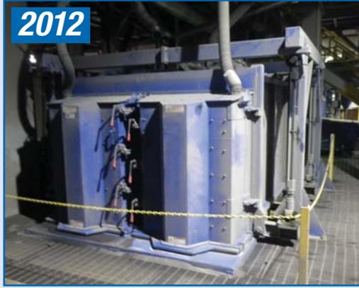
2012 Rotex Mineral Separator Model MM3180-3, 48' x 89" High Capacity, Twin Chamber Triple Deck Triplex Gyrotory Screener, s/n SO 38597/0
