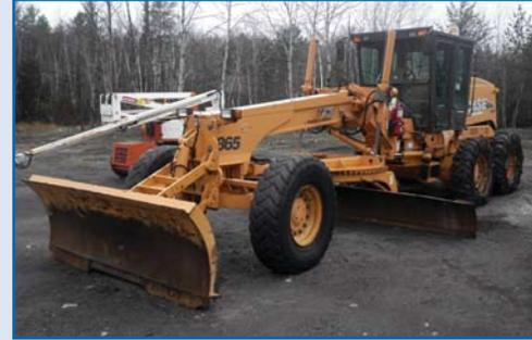
Case Model 865 Motor Grader, s/n 23804 w/ 14' Moldboard, 9' Henke Dozer Blade, PS Trans., 14R x 2400 Tires, Showing 7150 Hours
