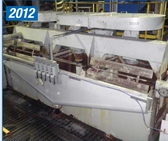
(4) 2012 Quinn Process Equipment Model QPEC #100 T-BR Flotation Machines c/w Double Froth Overflows and Froth Paddles with Drives & c/w Spencer Model 30103A3 Centrifugal Blower s/n 815558-F12
