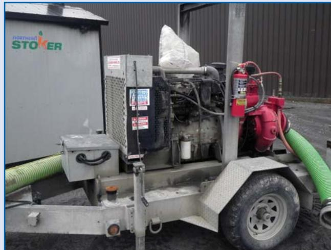
Claeson 6" Self-Priming Centrifugal Water Pump on S/A Chassis p/w 4 Cyl. Perkins Diesel
