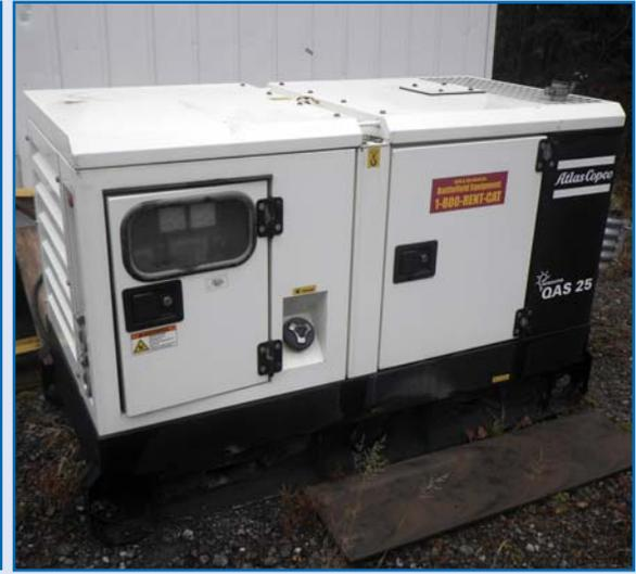
Atlas Copco Model QAS25KD-SKID, Skid Mount 20KW Generator, s/n HOP10097, 20KW/25KVA, 480/240/208V, 3 Phase
