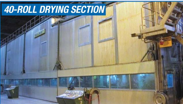
**7.2M VALMET** Paper Machine (New 1981) w/ Upgrades, 1387 MPM (4550 FPM), 37-59 GSM, 283" Trim, Dilution Headbox, Gap Former, Tri Nip Press w/ Shoe Press and Separate 4th Press, 7-Roll Unirun Section w/ Additional 40-Roll Drying Section, Metso SW800 Scanner (New in 2012), and Valmet Optireel, Line in Excellent Condition, Possible Conversion to Light Weight Liner Board Machine
