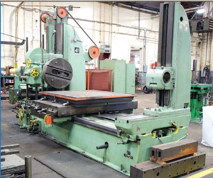
**ASQUITH 6" Floor Type Horizontal Boring Mill, 50 Taper Power Drawbar, Travels: X-240", Y-96", Z-60", Spindle Speed Range 1.5 - 600 RPM, Spindle Feed Rate .018 - 60 IPM, Fagor Innova 3 Axis DRO, 32" Dia. Facing Head, 96" x 96" Infeeding Power Rotary Table w/ Pendant, (120" x 180" Floor Plate) (May be sold separately) Threading, Full Pendant Controls, 30 HP, sn S20907.**
