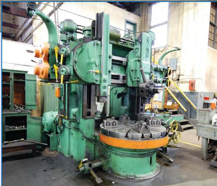
**SCHIESS** Model 2K 300/500 Vertical Boring Mill, Table Diameter 118.1", Swing 196.8", Horizontal Head Travel 102", Vertical Head Travel 66.9", Approx. Work Height Under Rail 78.74", 4 Jaw Chuck, Twin Swiveling Rams, 2 Sony 2 Axis DRO's, Dual Pendant Control, Operator Panel, .71 – 52.5 RPM, Threading, 40 HP, sn 73138
