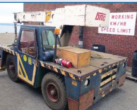
**BMC** Model IC80 1B Mobile Crane, Max 17,000 lb on Outriggers, Max 30', Up To 70 Degree, Cab, sn 813B
