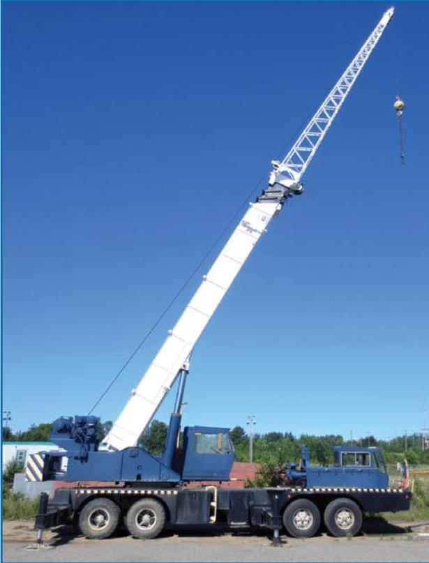
**GROVE** Industrial Tractor Crane Carrier Model 8450 G, sn BCIX5016LN 32180, 1974, GVWR 82,000 lb, Front & 1st Int Axles 18,000 lb, 2nd Int & Rear Axle 23,000 lb, 4,216 Miles, Grove Mobile Crane Model TMS 475 LP, Up To 100,000 lb Capacity, 142' Max Reach, 4 Stage Boom, 6' Outriggers, sn 32180
