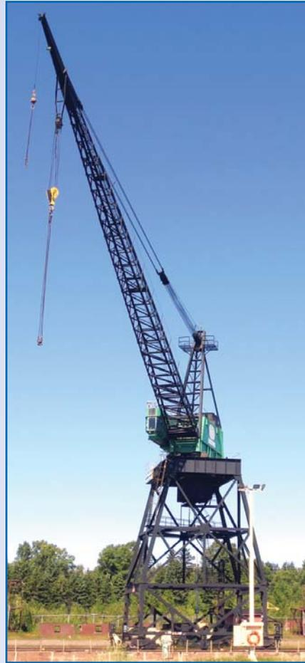
**COLBY** Mobile Gantry Crane, Model 240, 45 Ton Capacity, Radius Range 67' - 143', Up To 30 FPM, Plus 5 Ton Auxiliary Hoist at Any Radius, Up To 150 FPM, Cab Operated Full Control, Crane Smart Digital Readout, Hoist Room Monitor, Gantry Bridge Travel 110 FPM, Travels on Rail, Approx Max Wheel Load at Gantry 80,000 lb, Approx Crane Weight 250,000 lb, 550 V, sn 42121-45-MON-240
