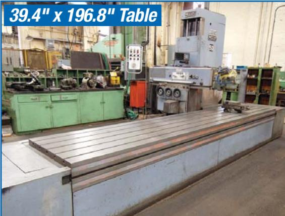
**MECOF** Model CS8 Travelling Column Universal Mill
