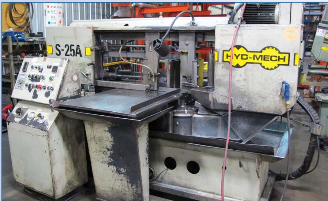
**HYD-MECH** S-25A automatic horizontal bandsaw with 18" x 27" capacity, hydraulic clamping s/n 90489141
