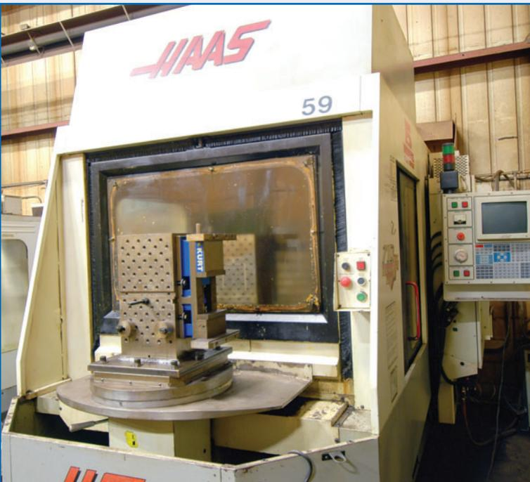
**HAAS HS-1 CNC HORIZONTAL MACHINING CENTER**
