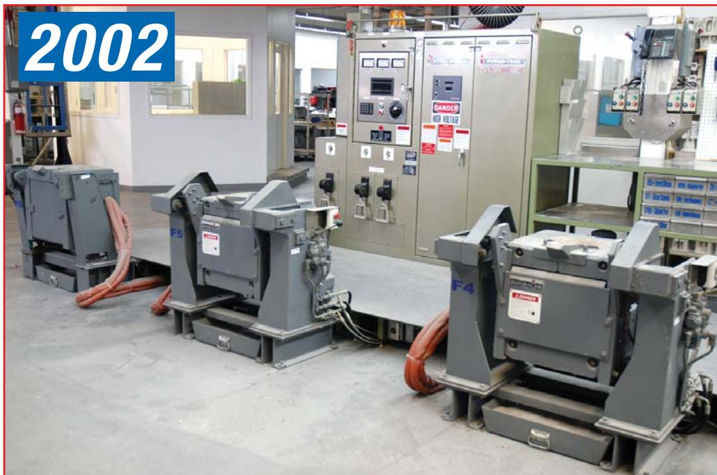
**INDUCTOTHERM** 175KW INDUCTION POWER SUPPLY, MODEL iPOWER-TRAK 175-30CR
