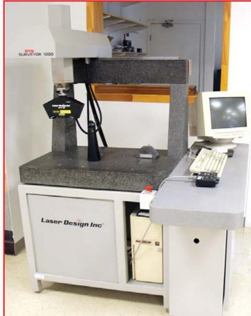
LASER DESIGN LASER CMM, MODEL SURVEYOR 1200
