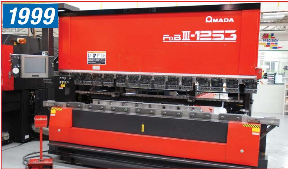
AMADA 10' X 138 TON HYD. PRESS BRAKE, MODEL Fx&B III-1253NT
