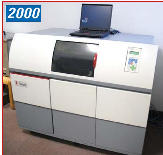
**3 D SYSTEM THERMOFORM THERMOJET SOLID OBJECT PRINTER**
