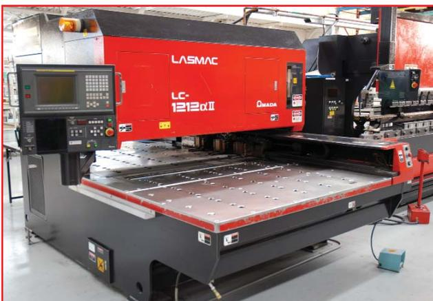
1995 **AMADA** Laser, Model LC-1212xII, Fanuc Oscillator Laser, Model C1500B, 1,500 Watts Max Laser Output, 50" Axis Travel, 65'/Min Cutting Speed, Rapid Axis Speed: X & Y-262'/Min & Z-196'/Min, 50" x 100" Max Sheet Size, .354" Max Sheet Thickness, 462 LBS Max Work Piece Weight, Fanuc Series 16-L Control, s/n 11212251
