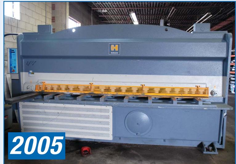
HACO SHEAR, 10' X 1/2" CAPACITY, MODEL HSL 3013
