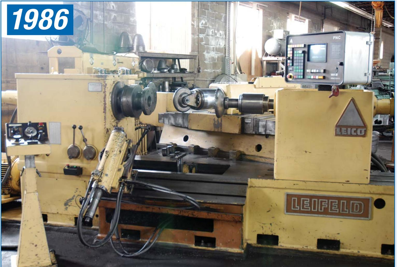
**LEIFELD** PNC 600, Max. Blank Size 47.24", Distance Between Centers 55.12", X Axis Travel – 19.69", Z Axis Travel – 27.56", Main Spindle Drive 40/30 HP, Hydraulic Pump Motor 33.5 HP, Slide Power Transverse (X) & Longitudinal (Z) 22,480 lbf (pound force), Tailstock Stroke 25.59", Ejector Stroke 15.75", Spindle Mount (Tool Adaptor) DIN 11, Including The Following Options: KA Unit, Material Support Device, Centering Unit, Roll Block System – Slide Lifting, 600V, Series 3/1, sn 10.1957.0
