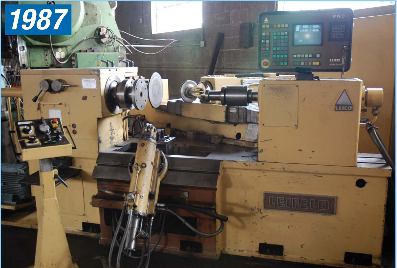
**LEIFELD PNC 450**, Max. Blank Size 35.43", Distance Between Centers 40.35", X Axis Travel – 12.20", Z Axis Travel – 19.69", Main Spindle Drive 25/15 HP, Hydraulic Pump Motor 28.5 HP, Slide Power Transverse (X) & Longitudinal (Z) 14,612 lbf, Tailstock Stroke 19.69", Ejector Stroke 11.81", Spindle Mount (Tool Adaptor) DIN 8, Including The Following Options: KA Unit, Material Support Device, Centering Unit, 600V, Series 20/1, sn 10.2224.0
