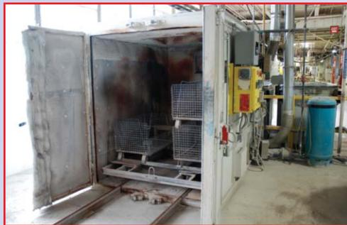
CONTROLLED PYROLYSIS FURNACE
