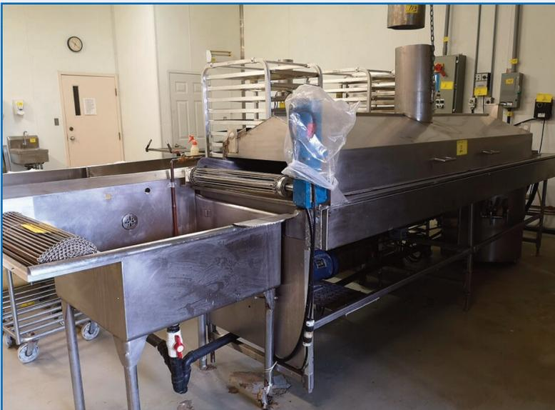
**POSS DESIGN 0011-24 CONTINUOUS COOKER, 40KW, 220V W/ COOKING/MIXING KETTLE & COOLING HOPPER, INFED CONVEYOR, CONTROLS, S/N 011**
