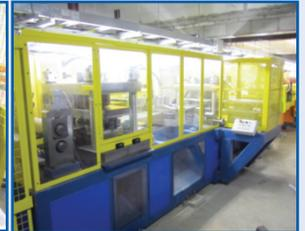
**DECOILER** Multiple Position Decoiler System – (5) Carousel 5,000 Lb Capacity Decoilers, 21" Mandrels, **STRAIGHTENER & FEEDER** 26"x36" Pinch Rolls, **FEEDER** 24" Width, **FLYING PUNCH & FIXED PUNCH** Roller Infeed Guide, 22.5"x5" Rolls
