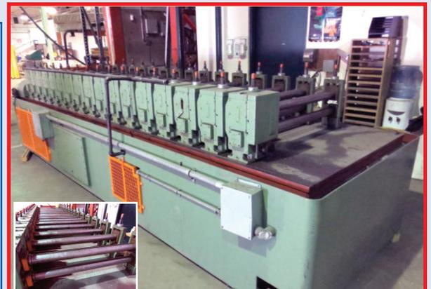
**ALSO AVAILABLE: ARDCOR** 17 Stand Rollformer, Model S10-21233, Vertical Centers 4-5-1/4", Horizontal Centers 10", Roll Space 33", Spindle Diameter 2.5", Table Size 56.5" x 200", Coolant Tank Cap 200 Gal, 40 HP, sn 90052. *This Rollformer Will Be Sold As A Separate Lot.*
