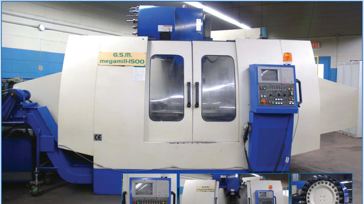
**GSM CNC VERTICAL MACHINING CENTER,
