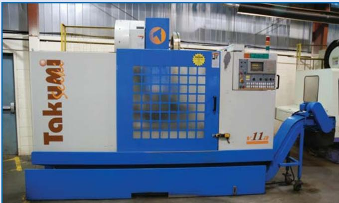
TAKUMI CNC VERTICAL MACHINING CENTER, MODEL V11A
