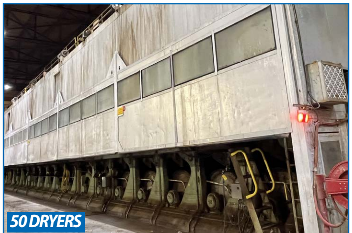
BLACK CLAWSON 178" Trim Paper Machine, 2200 Feet Per Minute, 480 Tons Per Day Max Output, 191" Slice Width, 195" Wire Cantilevered Fourdrinier, 50 Dryers (4 Sections), Super AUTOFLYTE 36" Reel, 187" Drum Face, MODULANT 186" Slitter Winder, B.T.H.B. 12"x191" Single Roll bunched Tube Headbox 9 PT Corrugated Medium Product, Travel from Right to Left s/n B-1160-1038
