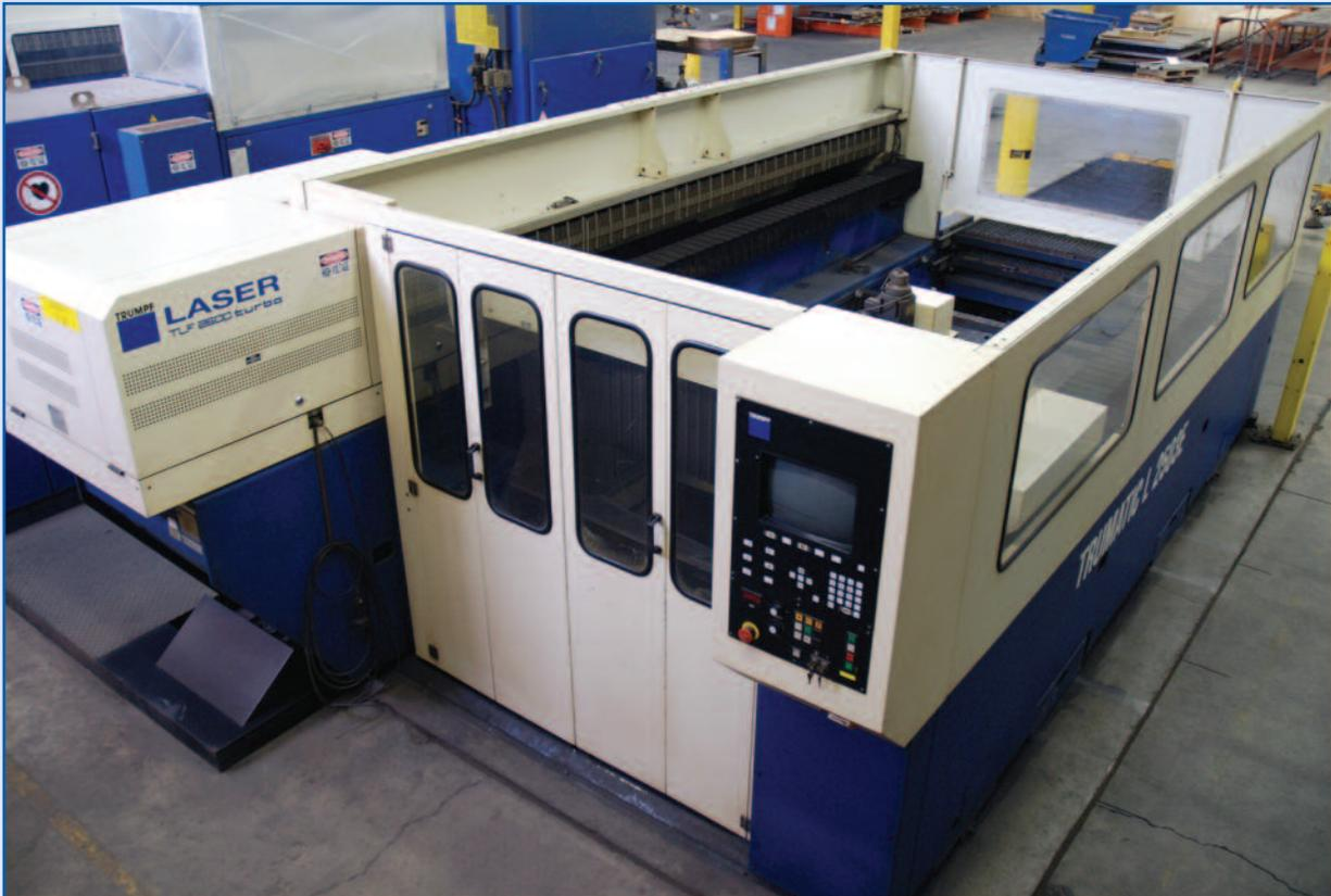
**TRUMPF** Laser Cutting System Model Trumatic L2503E, Trumatic Control, TLF 2600 Turbo Resonator, Chiller, Dust Collector, Auto Pallet Changer, Light Curtains. Laser Power 2600 W, Table 5'x10', Travels: X-61", Y-121", Z-4", 460V, 70Hz, sn 902914
