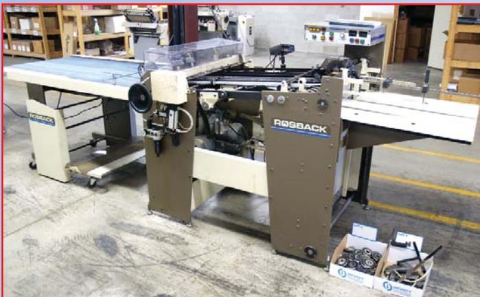
**ROSBACK MODEL 240 VACUUM PILE FED PERFORATOR, SCORER, CREASER, SLITTER**
