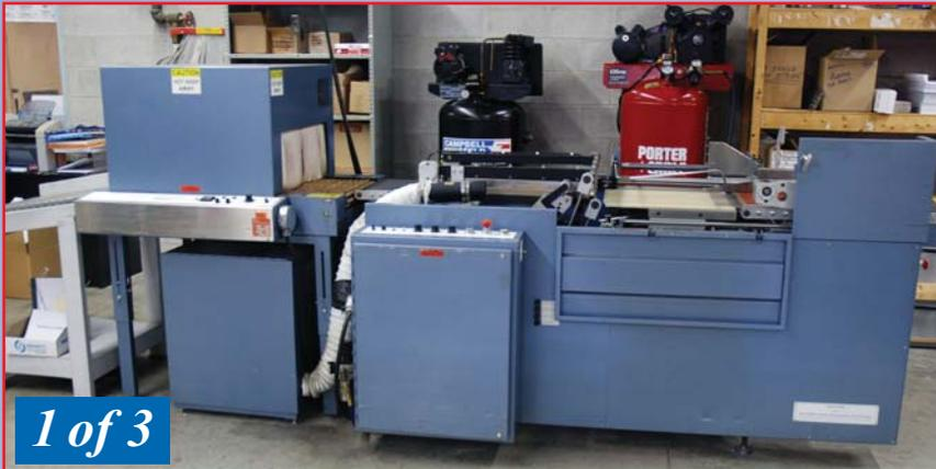
**RBS MODEL IALS 16"X20" AUTO FED L BAR SEALER, UNWIND STAND, ELECTRIC HOLE PUNCH, HEAT TUNNEL**
