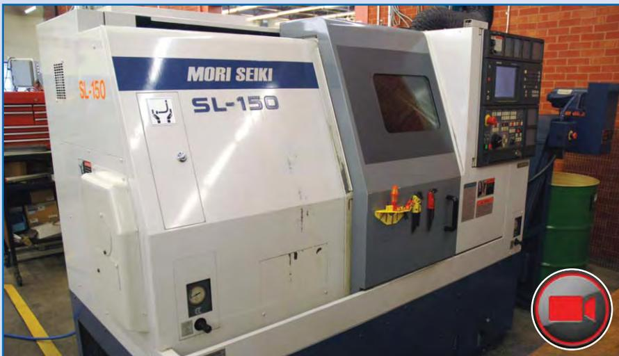
1998 **MORI SEIKI** Model SL 150/500, MSC500 CNC Control, Swing Over Bed 26.77, Swing Over Cross Slide 17.91", Distance Between Centers 22.05", Travels: X-9.06", Z-20.47", 12 Station Turret, Tailstock, Renishaw HPA Touch Probe, Kitagawa B206 6" Chuck, 50-5,000 RPM, Rapid Traverse X-708 IPM, Z-944 IPM, Chip Conveyor, 10 HP, sn 1027 (Excludes Aercology Air Filter). *View Video On Website!*
