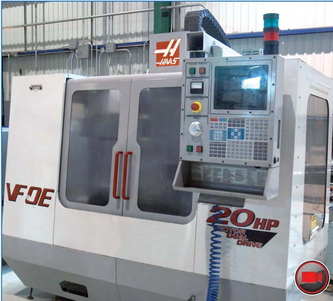
2000 **HAAS** CNC Lathe Model VF-0E, Travels: X-30", Y-16", Z-20", Table Size 30"x16", Cat 40, 7,500 RPM, Max Table Load 3,000 lbs, 20 HP, Rigid Tapping, 4th Axis Ready, Quick Code, Brushless Servos, sn 22839 (Dorion, PQ).
