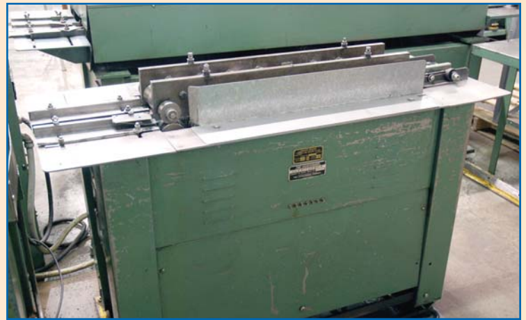
CLEATFORMER MODEL 22SS, TRIPLEX: FLAT S, DRIVE CLEAT, ACME LOCK, 22 GAUGE CAPACITY
