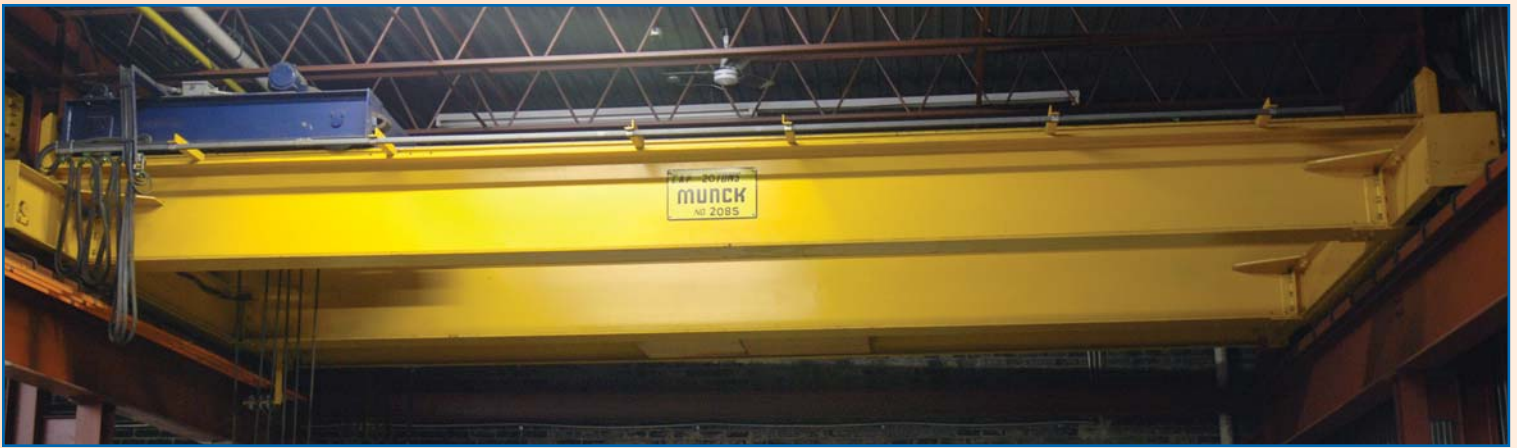
MUNCK 20 TON CRANE, 26'8" SPAN
