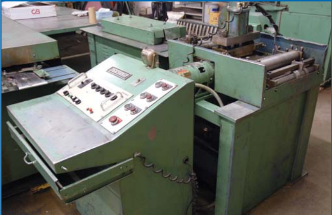
LOCKFORMER ELECTRO-FEED BATCH CUTTER, UP TO 12" CAPACITY, PLUS LOCKFORMER COIL FEEDER, KEEPER ARMS (BATCH CUTTER CURRENTLY FEEDS BOTH STANDING S AND TRIPLEX)
