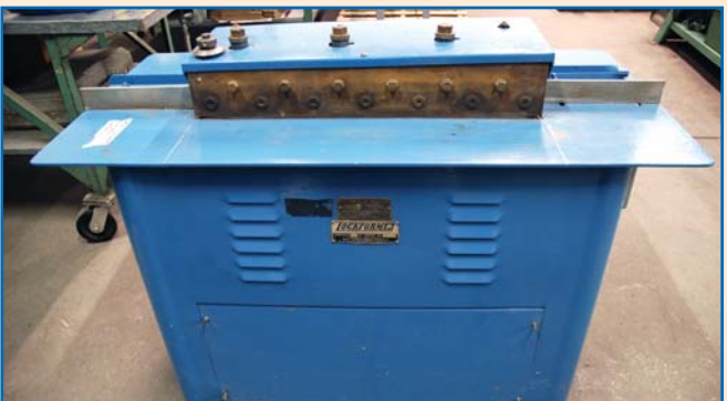
LOCKFORMER PITTSBURGH 24-16 GAUGE, DRIVE CLEAT ROLLS
