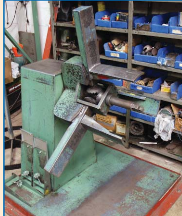
LOCKFORMER ELECTRO-FEED BATCH CUTTER, UP TO 12" CAPACITY, PLUS LOCKFORMER COIL FEEDER, KEEPER ARMS (BATCH CUTTER CURRENTLY FEEDS BOTH STANDING S AND TRIPLEX)
