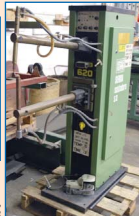
SERRA SOLDADURA MODEL SP 620, 20 KVA SPOT WELDER
