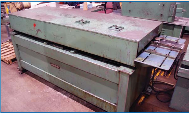
LOCKFORMER REINFORCED STANDING S CLEAT AND STANDING S, MODEL # 20
