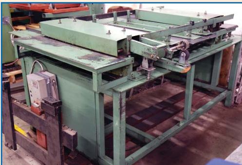
LOCKFORMER DUPLEX DUAL SIDED BUTTON LOCK MACHINES
