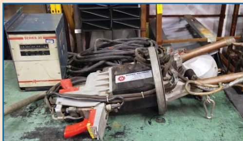
TECNA 22 KVA PORTABLE SPOT WELDER
