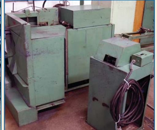
LOCKFORMER TURN & VAIN / DUCT TURN
