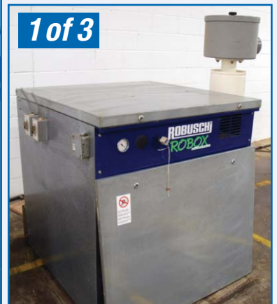
ROBUSCHI ROBOX EVOLUTION BLOWERS, MODEL ES 45/2V-RVV80
