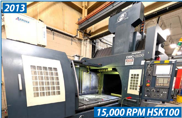
2013 JOHNFOR DMC-2100H CNC BRIDGE TYPE VERTICAL MACHINING CENTER. THERMAL GROWTH COMPENSATION FOR SPINDLE. LOOK AHEAD EXTENDED (1000 BLOCK LOOK AHEAD), HEIDENHAIN LINEAR SCALES ON XYZ
