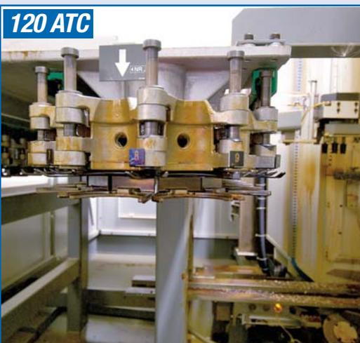
2008 **DECKEL MAHO DMC 100U Duo Block** CNC 5-Axis Machining Center, RS4 (6) Pallet Changer, s/n 1148 000165 3, DMG 3D Heidenhain i TNC530 CNC Control, 39-1/2" x 31-1/2" Pallets, Travels: X-39.37" (1000mm), Y-49.21" (1250mm), Z-39.37" (1000mm), HSK100 Spindle, Speeds to 12,000 RPM, (120) ATC, Dual Auger Chip Recovery, Chip Conveyor, Rotoclear S Window System, Coolant System, Coolant Through Spindle, 7,857 Power On Hours, 2,480 Run Time Hours (Approx. \$1.3 Million New)
