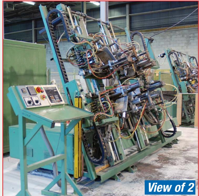
**URBAN** MODEL AKS 1400 ETL AUTOMATIC 4 HEAD BUTT WELDING MACHINE
