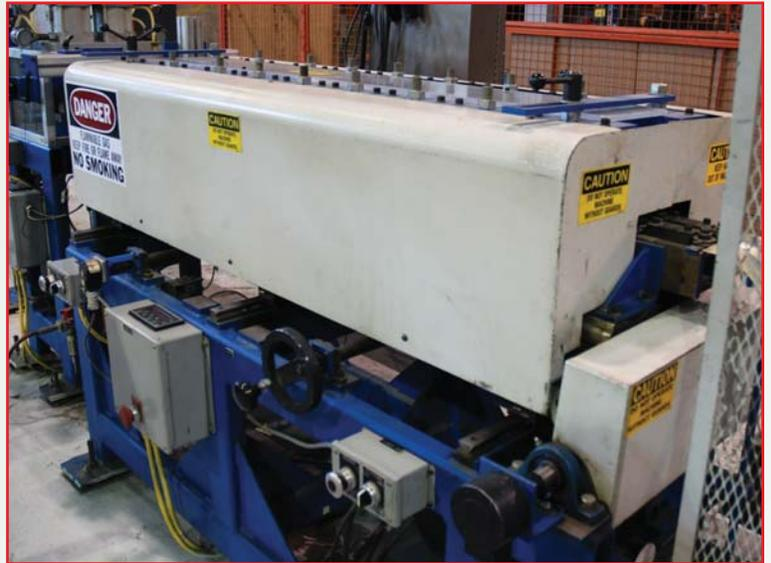
9 STAND ROLL FORMER, VIDEOJET EXCEL HIGH RESOLUTION INJET PRINTER, CUT-OFF (STATIC)
