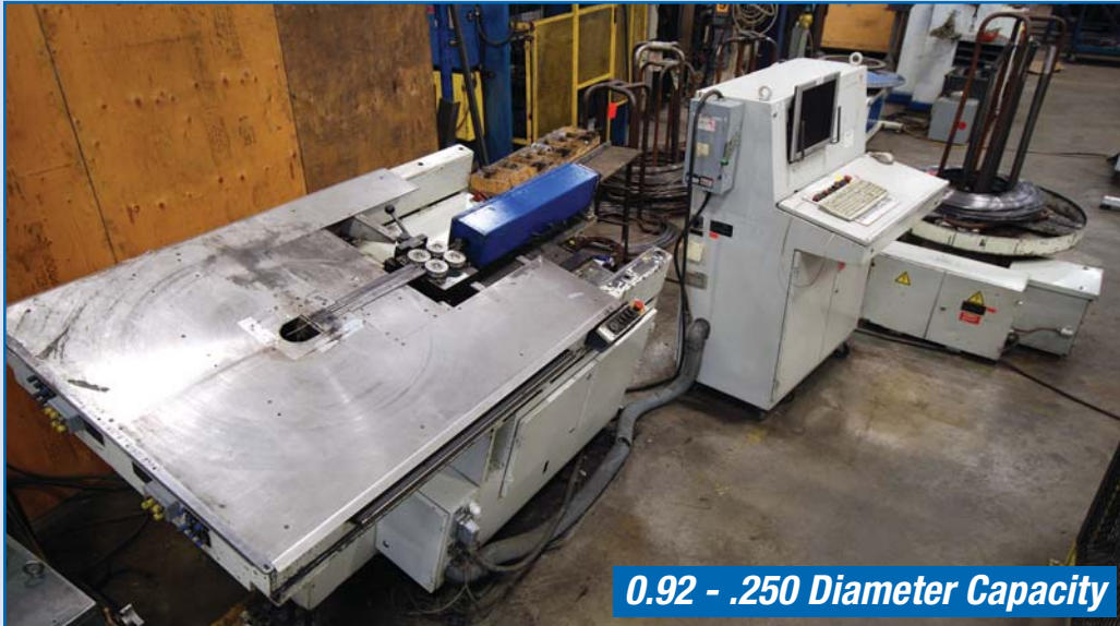
WAFIOS BM 3-2 D, 3-Axis, CNC Wire Bender, Cutoff, Assorted Dies .092 - .250 Dia. Cap, 262 ft/main feed, sn 27551007, Plus Wafios Automatic Uncoiler Model AHL 41 B, 48" Bed, sn 27919354
