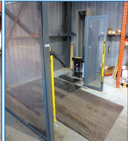
SAMUEL SLP175 Pallet Wrapper With Cage Enclosure And Light Curtains s/n 1222031425
