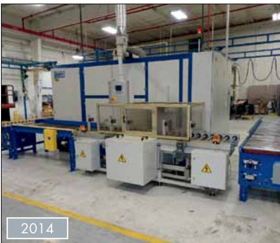
DURR ECOCLEAN AQUEOUS PARTS CLEANER/ WASHER, MODEL UNIVERSAL 81W
