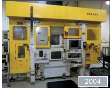
MITSUBISHI 6-AXIS CNC GEAR HOBGING MACHINE, MODEL GHD10A
