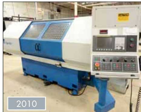
SUPERTEC CNC CYLINDRICAL GRINDER, MODEL G31A-50CNC
