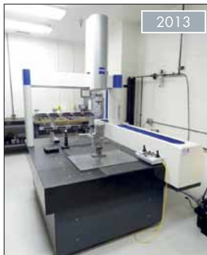
ZEISS CNC COORDINATE MEASURING MACHINE, MODEL CONTURA G2
