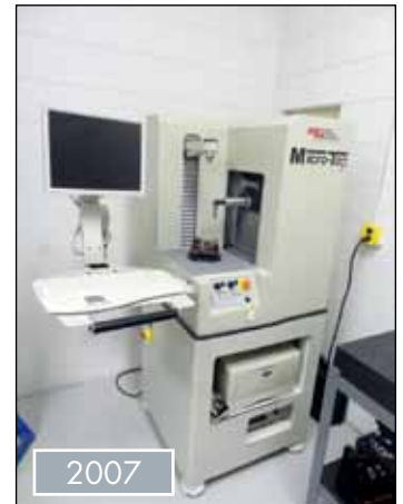
M&M PRECISION SYSTEMS MICRO-PRO 34587-B08 GEAR ANALYZER
