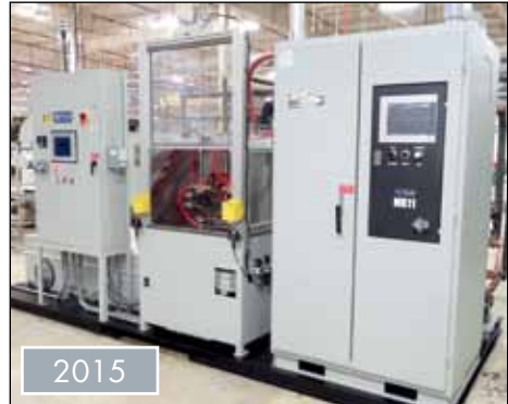
PILLAR INDUCTION HEAT TREAT SYSTEM, MODEL AB7102-114/MK 11, 200KW
