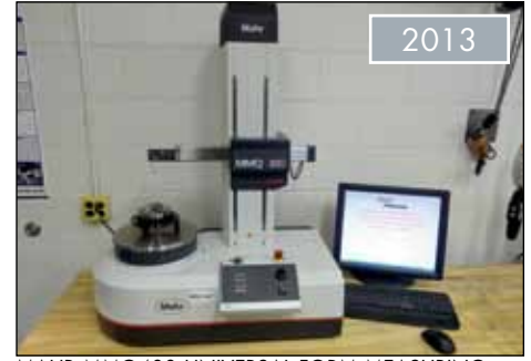
MAHR MMQ400 UNIVERSAL FORM MEASURING MACHINE, ROUGHNESS CHECKING GAGE; WITH MAHR T7W HEAD
