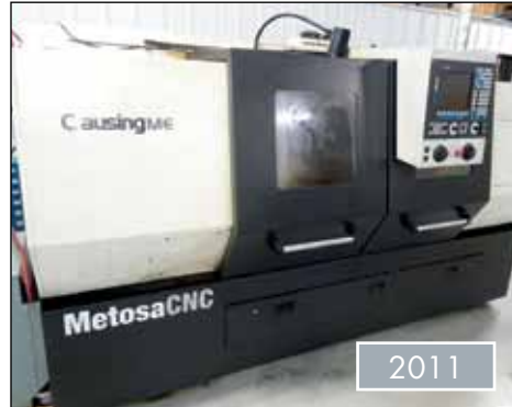
CLAUSING METOSA MC17 CNC LATHE
