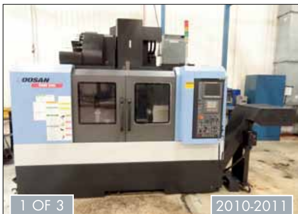
DOOSAN CNC VERTICAL MACHINING CENTER, MODEL DNM500, KOMO 4TH AXIS
