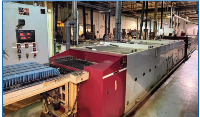
MORTON/ADVANCED CHEMILL SYSTEMS STRIP/ETCHING/STRIP LINE - RESIST STRIPPER RS 67, TIN STRIPPED TS 430, ETCHER MODEL ULTRA ETCH 20, TRIPLE CASCADE RINSE MODULE
