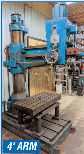
KITCHEN & WADE 36E26 RADIAL DRILL
