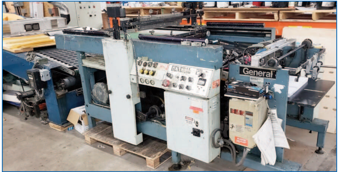
GENERAL SHEET FED SCREEN PRESS W/ UV DRYER
